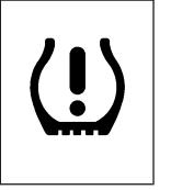
As an added safety feature, your vehicle has been equipped with a tire pressure monitoring system (TPMS) that illuminates a low tire pressure telltale when one or more of your tires is significantly under-inflated.
